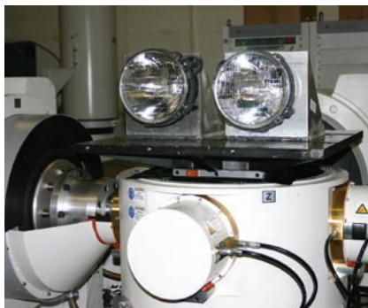
FIGURE 1: An array of three electrodynamic shakers simultaneously vibrates test items north-south, east-west, and up-down. (Courtesy Spectrum Technologies, Inc., Redford, Michigan)
